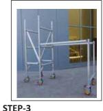
Fit caster wheel in one rung frame and then attached the frame with two horizontal to three rung span frames. Make sure hook facing outside from inside.
